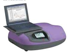
A robust and simple to use single beam scanning instrument for general laboratory measurements that also includes software routines for nucleic acid measurements and enzyme kinetics.
